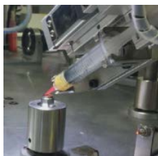
Figure 8. Crimped inner wall needle positioning
