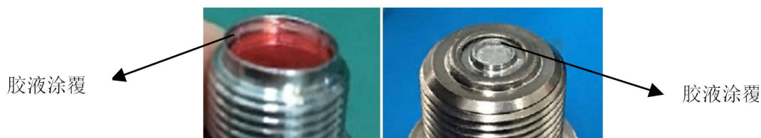
Figure 10. Gluing effect of inner wall of igniter winding edge 图 10. 点火器卷边内壁涂胶效果图
