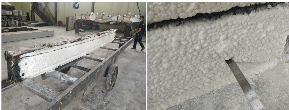
Figure 4. Foaming situation of fireproof coating after fire resistance test
