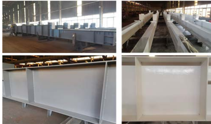
Figure 5. Pre-painting fireproof coating in the factory 图 5. 钢构件工厂预涂装防火涂料
