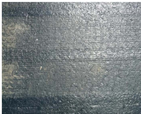
Figure 8. Wheel track after rolling 图 8. 车辆碾压后产生轮迹
