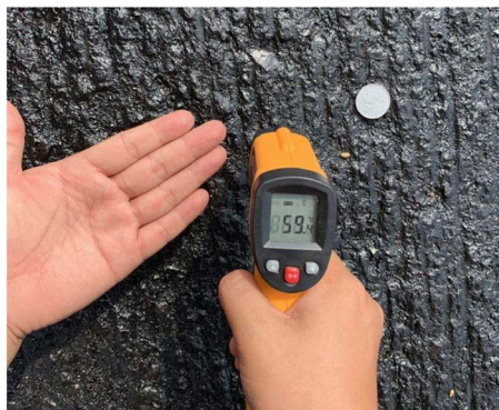
Figure 7. No hand sticking after demulsification 图 7. 破乳后无粘手现象
