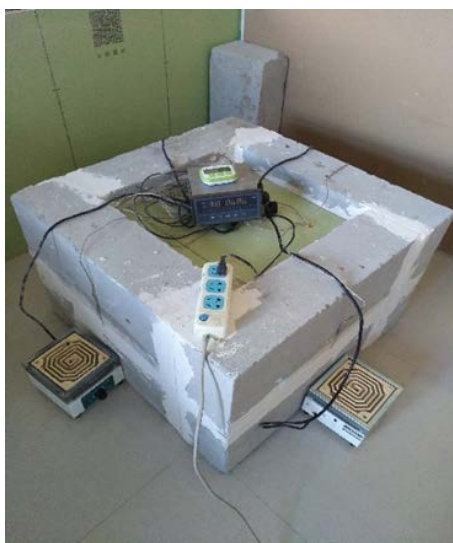
Figure 5. The simulation device for measuring thermal insulation performance 图 5. 保温隔热性能模拟测定装置
