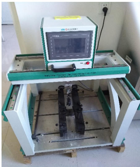
Figure 4. The device for measuring bond strength 图 4. 拉拔强度测定装置
