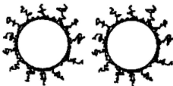
Figure 8. Schematic diagram of steric hindrance stabilization mechanism
