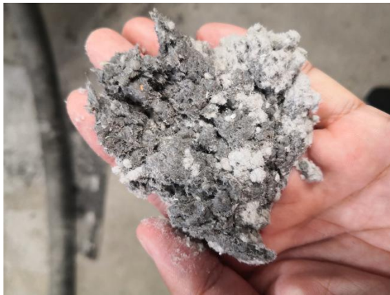
Figure 12. Sampling effect of hot warehouse mineral and wood fiber after mixing 图 12. 热仓矿料和木质纤维拌和后取样效果
