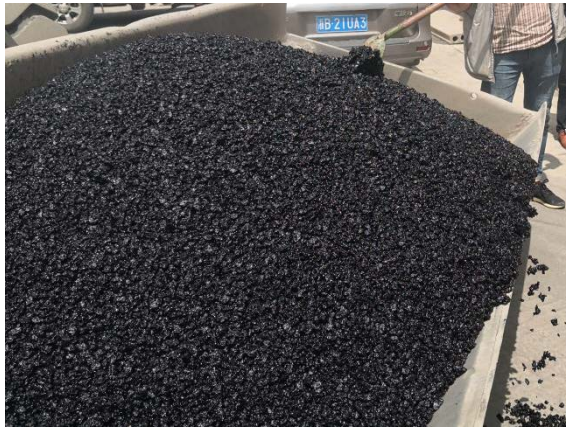
Figure 11. Trial mixture “rich oil” 图 11. 试拌混合料“富油”
