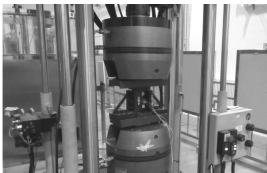
Figure 4. Compression test device after impact 图 4. 冲击后压缩试验装置
