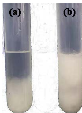
Figure 8. Photographs of (a) pure \text{Na}_2\text{HPO}_4 \cdot 12\text{H}_2\text{O} and (b) composite phase change material after crystallization for 0.5 h
