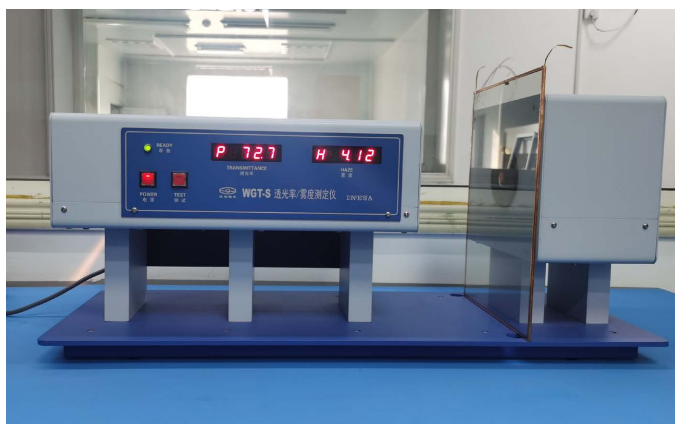
Figure 5. Transmittance and haze test results of 15-inch electric heating shielding glass 图 5. 15 吋电加热屏蔽玻璃透过率、雾度测试结果
