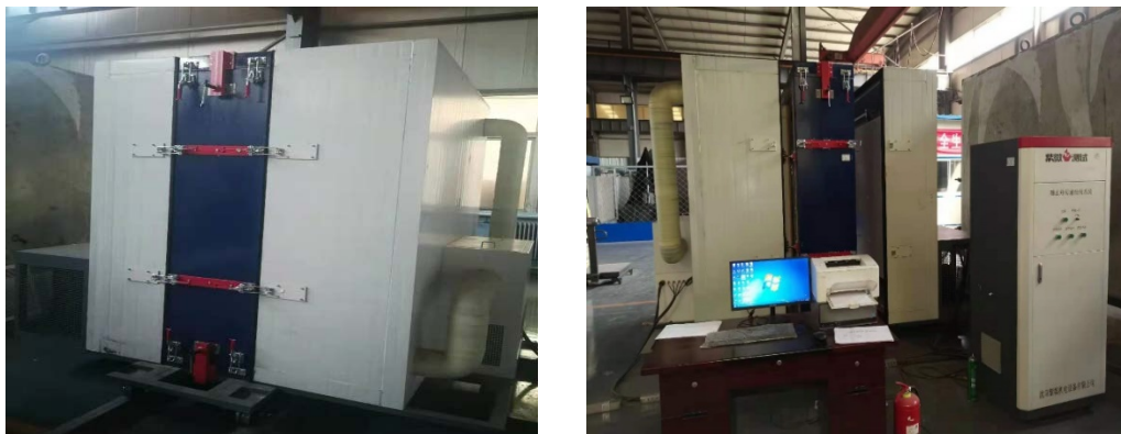
Figure 1. Steady-state heat transfer property test system 图 1. 稳态热传递性质测试系统
