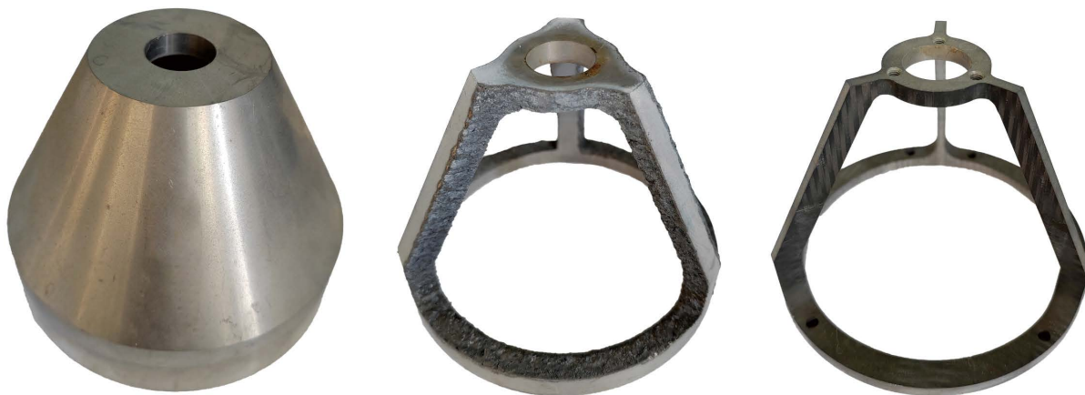
Figure 12. Arc discharge-mechanical milling combined machining process of SiC p /Al structural parts; (Left) Blank material; (Medium) High power arc discharge rough machining; (Right) Low arc discharge semi-finishing and digital milling machining 图 12. SiC p /Al 结构件电弧放电-机械铣削组合加工过程；(左) 坯料；(中) 高功率电弧放电粗加工；(右) 低电弧放电半精加工和数控加工
