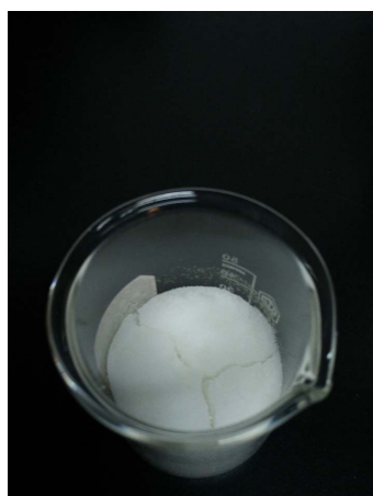
Figure 2. The state of polymer waste oil absorbent after oil absorption 图 2. 高分子材料废油吸收剂吸油后的状态
