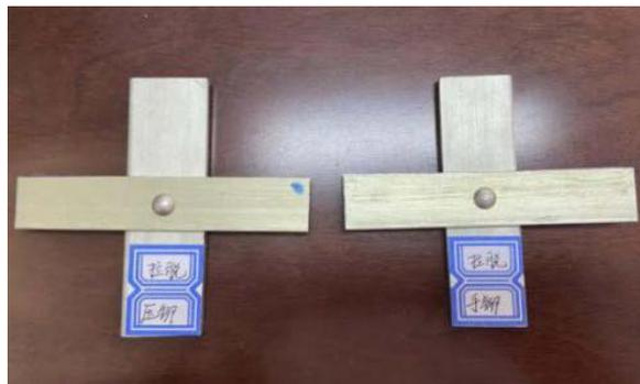
**Figure 4.** The pull off sample
