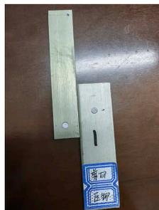
Figure 3. The schematic of rivet nail breakage after the shear test
