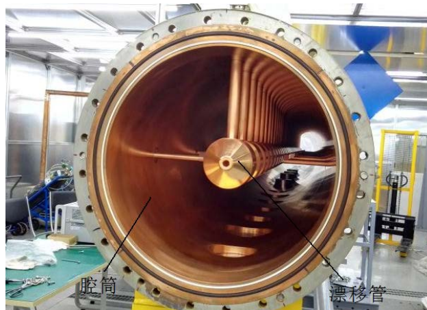
Figure 1. Structural of drift tube linac 图 1. 漂移管直线加速器实物图
