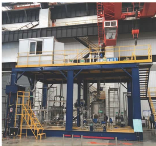
Figure 5. Spent resin steam reforming pilot test rig 图 5. 废树脂蒸汽重整中试试验台架[13]
