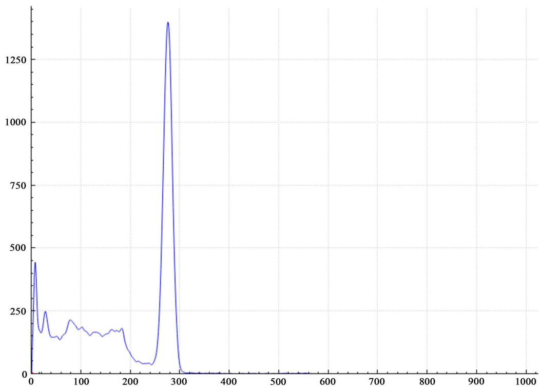
Figure 4. Smoothed energy spectrum using the five-point center of gravity method 图 4. 五点重心法光滑后能谱图
