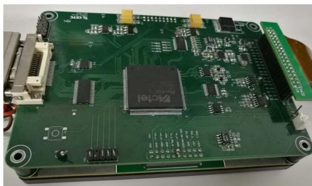
Figure 6. Photo of drive and signal processing circuit
