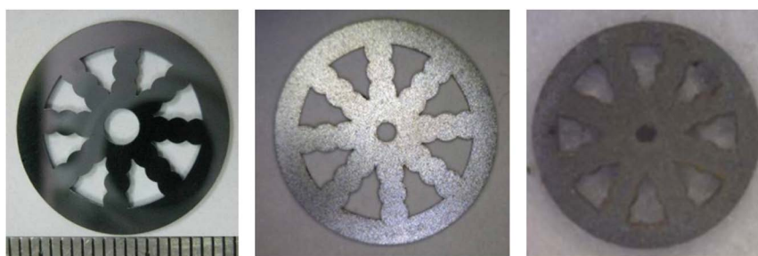
Figure 6. Laser cutting 0.6 mm, 0.38 mm, 0.18 mm thick monocrystalline silicon 图 6. 激光切割 0.6 mm、0.38 mm、0.18 mm 厚单晶硅
