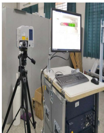
Figure 4. Vibration measurement with laser 图 4. PSV-500 激光测振仪
