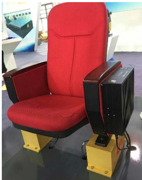
Figure 7. Active seat vibration reduction system prototype 图 7. 座椅主动减振系统实物图
