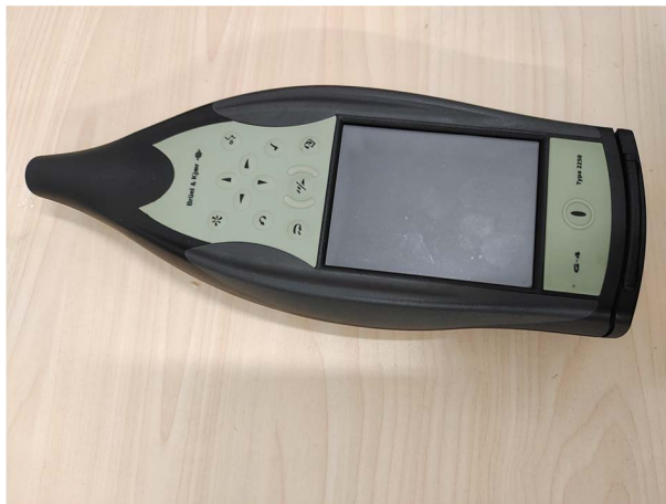
Figure 11. B-K Acoustic Acquisition Analyzer 图 11. B-K 声学采集分析仪
