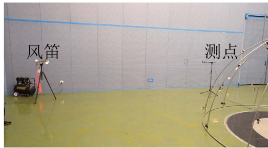
Figure 14. The test microphone is placed in air whistle 45° extension line 图 14. 传声器置于风笛 45°延长线测试
