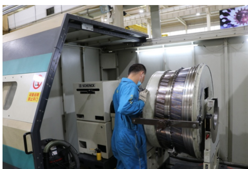
Figure 1. Assemble the fan rotor with heavy screws
