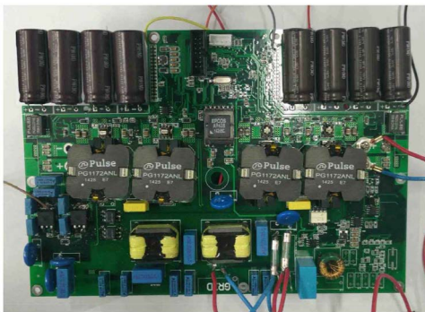
Figure 14. Experimental prototype of the dual-channel micro-inverter
