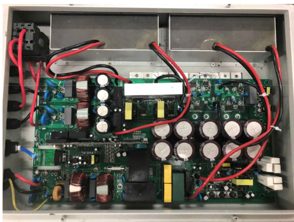
Figure 16. Experimental prototype of the single-phase grid-connected inverter 图 16. 5 kW 单相并网逆变器样机
