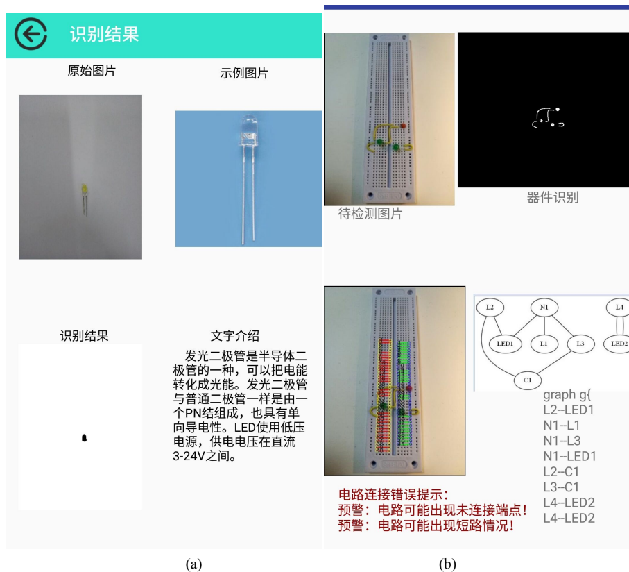
Figure 4. Examples of system usage effects; (a) examples of automatic component identification; (b) examples of automatic recognition of breadboard function circuit
