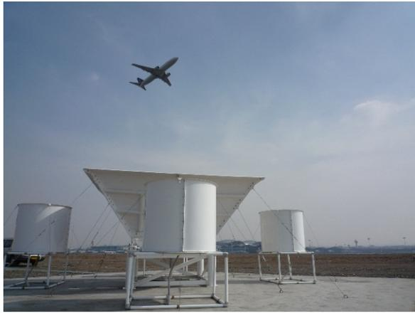
Figure 1. Wind profile radar
