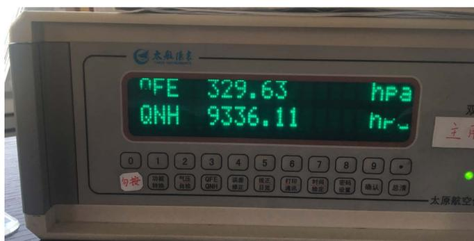
**Figure 1.** Display of vibration cylinder barometric malfunction**图 1.** 振筒气压仪故障显示
