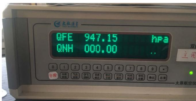
**Figure 2.** Display of vibration cylinder barometric malfunction**图 2.** 振筒气压仪故障显示
