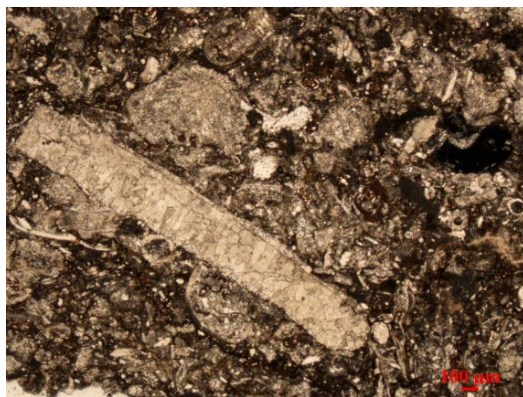
Figure 4. Micrite bioclastic limestone, the first member of Qixia Formation, showing algae and foraminifera
