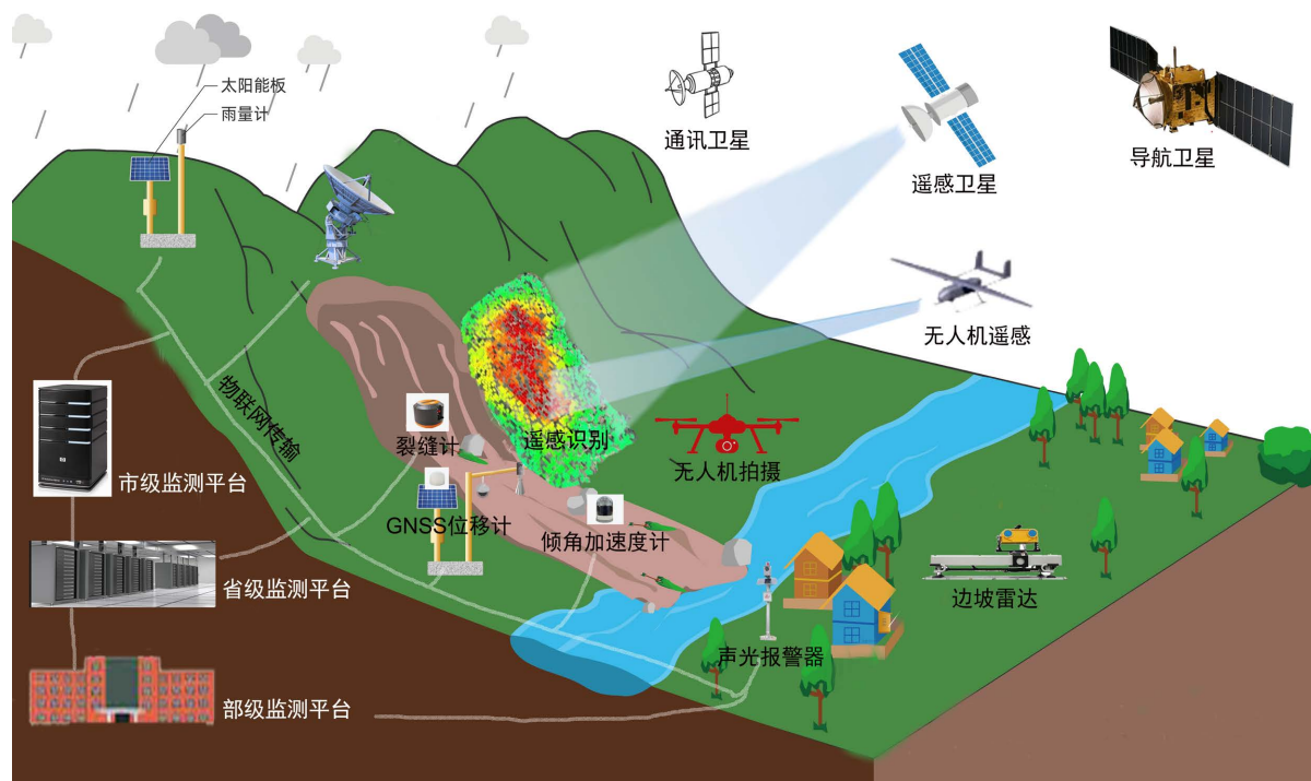
Figure 1. Integrated monitoring and early warning system for geological disasters 图 1. 地质灾害空地一体化监测预警体系
