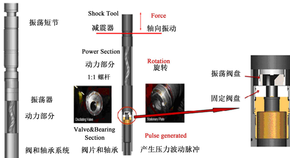
Figure 4. Schematic diagram of hydraulic oscillator structure
