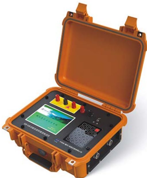
Figure 1. DUK-4 high-density electrical mainframe used to collect data
