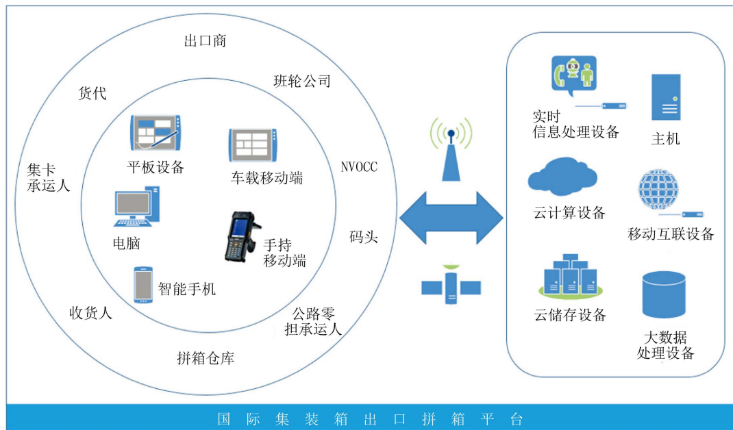
Figure 3. Hardware architecture of the intelligent information system 图 3. 智能化信息系统硬件构架
