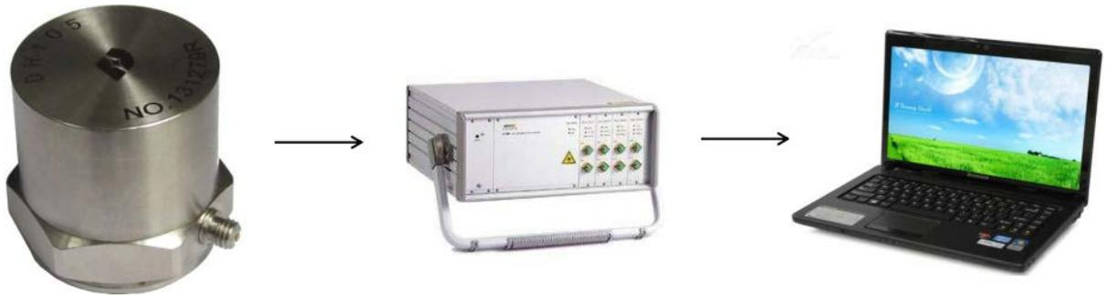
Figure 1. Measurement system for vibration signals
