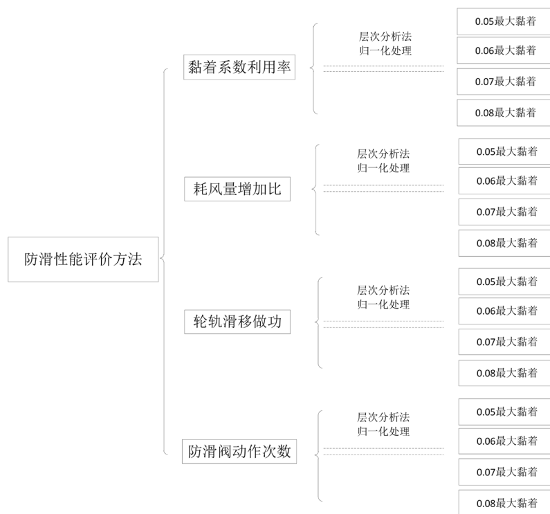
Figure 2. Schematic diagram of performance evaluation method for WSP system 图 2. 防滑系统性能评价方法示意图
