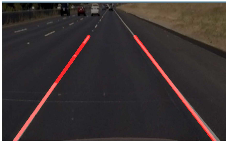
Figure 3. Result of lane line fitting detection
