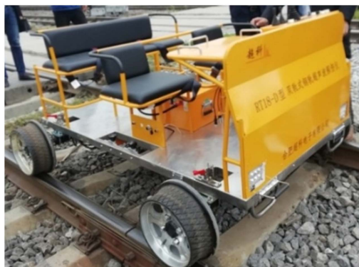
Figure 1. Rail inspection trolley
