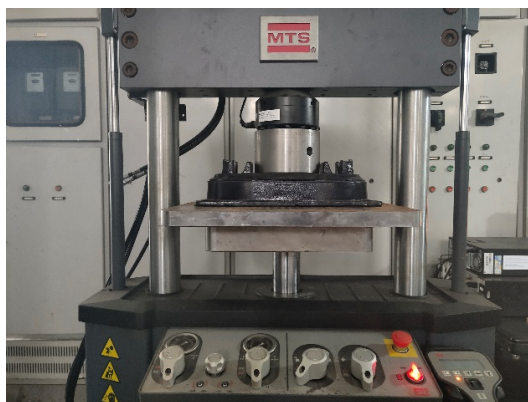
Figure 2. Test equipment of the track damper vertical stiffness
