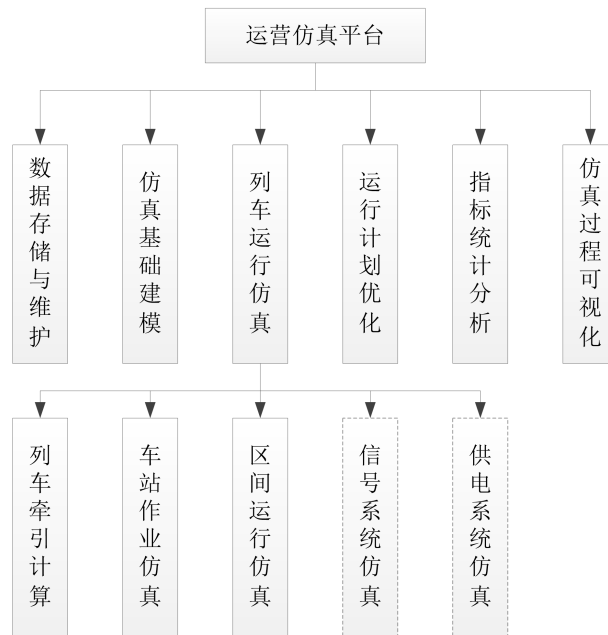
Figure 1. Schematic diagram of the functional structure of the simulation platform for train groups
