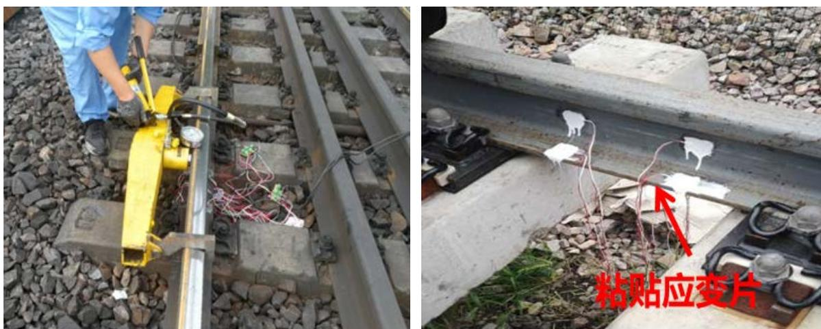
Figure 12. Field diagram of dynamic response test
