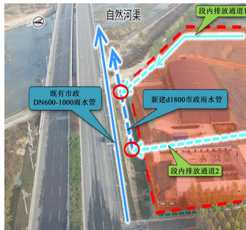
Figure 6. Case of rainwater flowing into natural river in vehicle base 图 6. 车辆基地雨水接入自然河渠案例
