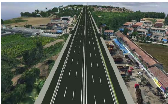
Figure 3. Highway elements acquisition based on UAV tilt photography
