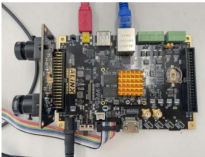
Figure 10. ZYNQ7020 hardware connection diagram 图 10. ZYNQ7020 硬件连接图
