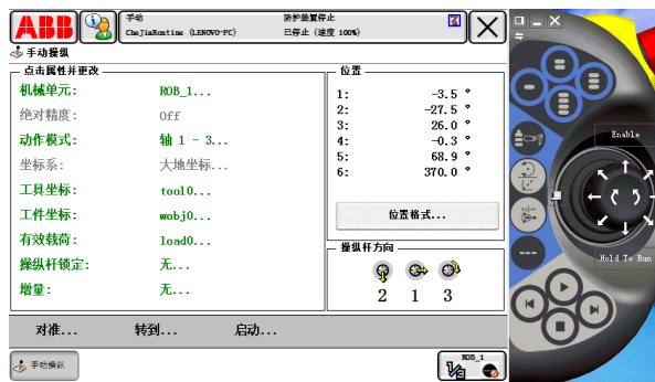
Figure 7. Setting tool (workpiece) coordinates and payloads 图 7. 设置工具(工件)坐标和有效载荷
