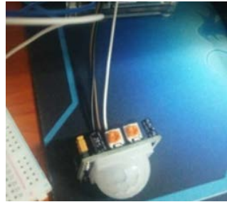
Figure 4. HC-SR501 type pyroelectric infrared switch 图 4. HC-SR501 型热释电红外开关
