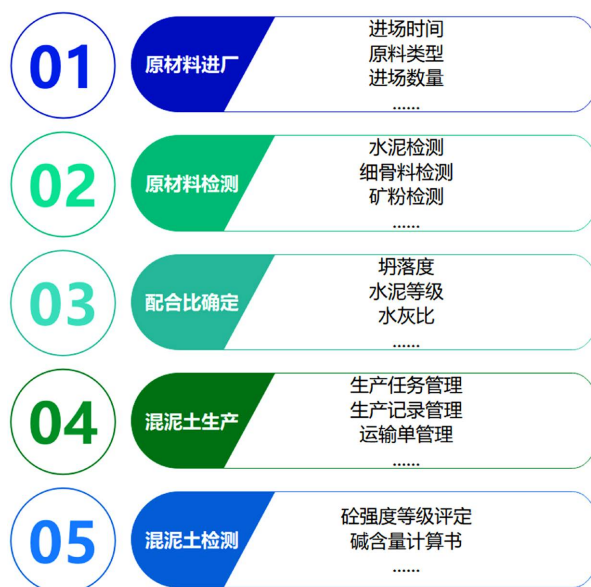
Figure 2. Concrete production process
