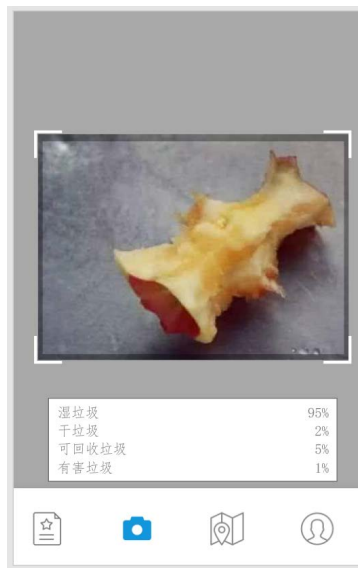
Figure 7. Recognition results 图 7. 识别结果
