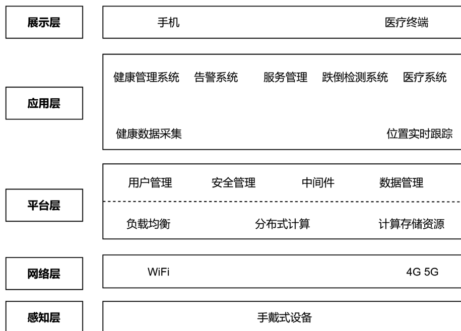
Figure 4. Architecture of health monitoring cloud platform
