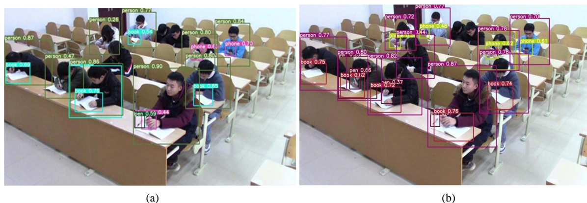
Figure 8. Comparison of detection results of occlusion small targets by network before and after improvement. (a) CBL_Triplet structure diagram; (b) Improved YOLOv5s detection results
