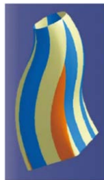
Figure 12. AFP path generated by CAD/CAM System developed by Xi'an Jiaotong University
