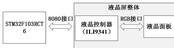
Figure 11. LCD control block diagram
